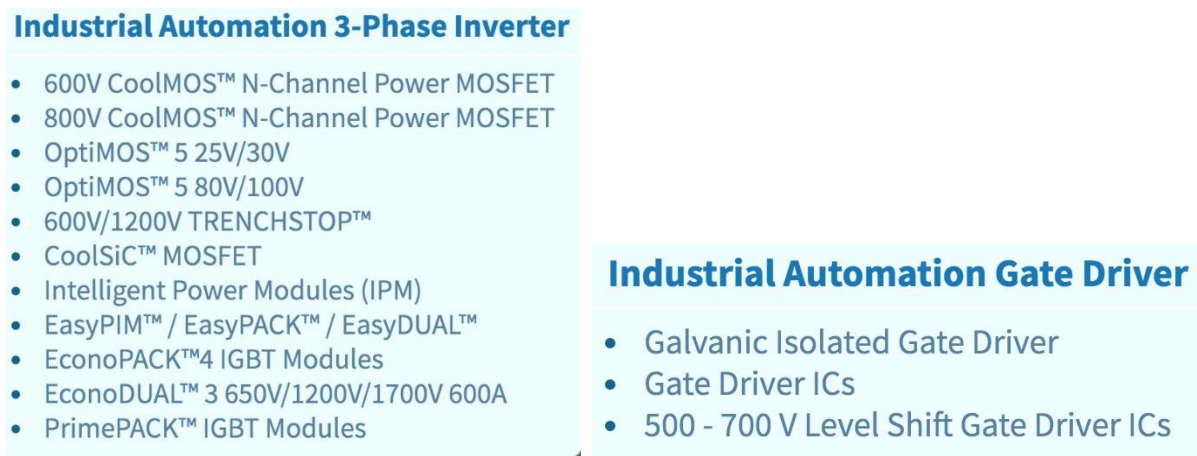
Fig. 13. Recommended available three-phase inverter options (left) and input driver control options (right) for three-phase inverter power circuits
